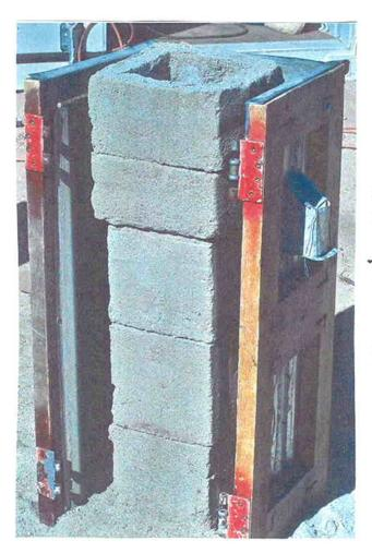
THREE (3) 8" x 8" x 8" x 8" BLOCKS AND TWO (2) 10" X 10" X 5" BLOCKS COMPLETE THE CAVITY. THE FILL BLOCK MATERIAL IS REMOVED DRY WITH A HARD NARROW TOOL
