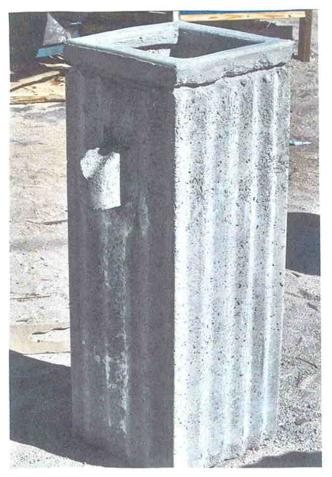
BLOCK, ALLOW 24 HOURS FOR CONCRETE TO SET. TILT MOLD AWAY FROM SPONT TO CLEAR BLEEDER TUBE
